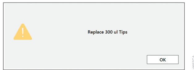
Figure 25. Insufficient tips on the system to complete a method. In the event that all tips of a given tip type are consumed during a run, the instrument will pause and unlock the door. Open the door, load more tips of the indicated type on the tip and plate carrier, close the door and press OK to resume processing.
