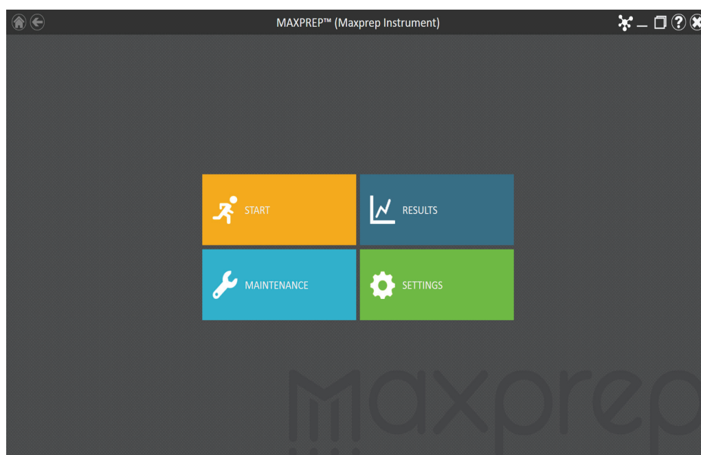
Figure 1. Maxprep® software 'Home' screen. From the Maxprep® software 'Home' screen, select the Start button to begin the process of running a method.
